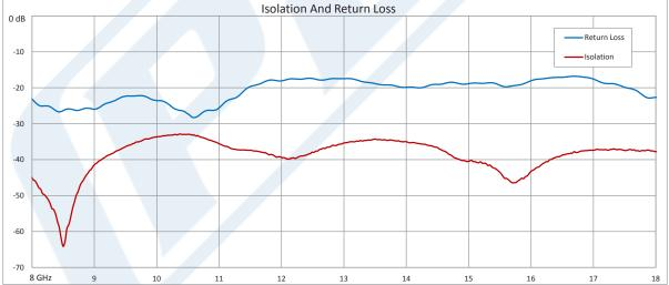
Click the following link (or enter part number in "SEARCH" on website) to obtain additional part information including price, inventory and certifications: Dual Junction Isolator With 32 dB Isolation From 8 GHz to 18 GHz, 5 Watts And SMA Female PE83IR1023
