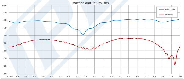
Click the following link (or enter part number in "SEARCH" on website) to obtain additional part information including price, inventory and certifications: Dual Junction Isolator With 36 dB Isolation From 4 GHz to 8 GHz, 10 Watts And N Female PE83IR1020
