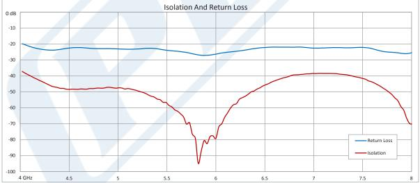
Click the following link (or enter part number in "SEARCH" on website) to obtain additional part information including price, inventory and certifications: Dual Junction Isolator With 36 dB Isolation From 4 GHz to 8 GHz, 10 Watts And SMA Female PE83IR1019
