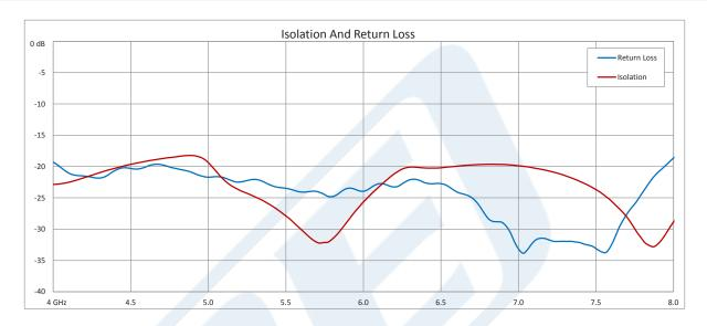
High Power Isolator With 18 dB Isolation From 4 GHz to 8 GHz, 50 Watts And N Female from Pasternack Enterprises has same day shipment for domestic and International orders. Our RF, microwave and millimeter wave products maintain a 99% availability and are part of the broadest selection in the industry.
