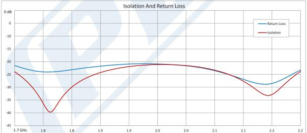
Click the following link (or enter part number in "SEARCH" on website) to obtain additional part information including price, inventory and certifications: High Power Isolator with 20 dB Isolation from 1.7 GHz to 2.2 GHz, 100 Watts and N Female PE83IR1003
