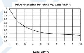
Power Handling Chart and Derating Curves based on the following Test and Environmental Conditions: Ambient temperature: 20 - 25°C
