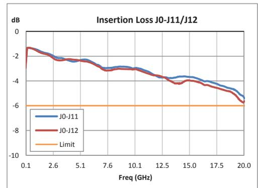
Click the following link (or enter part number in "SEARCH" on website) to obtain additional part information including price, inventory and certifications: [Absorptive SP12T PIN Diode Switch Operating From 100 MHz to 20 GHz Up to +27 dBm and SMA PE71S2034](#)
