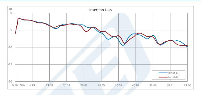
Click the following link (or enter part number in "SEARCH" on website) to obtain additional part information including price, inventory and certifications: Absorptive SPDT PIN Diode Switch Operating From 100 MHz to 67 GHz Up to +27 dBm and 1.85mm PE71S2026
