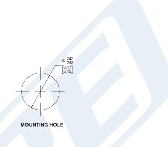
Click the following link (or enter part number in "SEARCH" on website) to obtain additional part information including price, inventory and certifications: Slide-On BMA Plug Bulkhead to TNC Male Cable Using RG316 Coax PE3C4947
