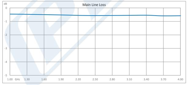
Click the following link (or enter part number in "SEARCH" on website) to obtain additional part information including price, inventory and certifications: Directional 10 dB SMA Coupler From 1 GHz to 4 GHz Rated to 50 Watts PE2209-10
