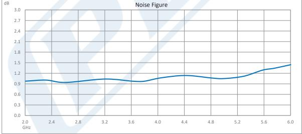
Click the following link (or enter part number in "SEARCH" on website) to obtain additional part information including price, inventory and certifications: Input Protected Low Noise Amplifier, 2 GHz to 6 GHz, 1 Watt RF Input Power, 40 dB Gain, 1.2 dB Noise Figure, 12V, SMA PE15A63019
