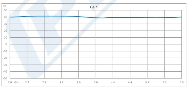
Click the following link (or enter part number in "SEARCH" on website) to obtain additional part information including price, inventory and certifications: Input Protected Low Noise Amplifier, 2 GHz to 6 GHz, 1 Watt RF Input Power, 40 dB Gain, 1.2 dB Noise Figure, 12V, SMA PE15A63019
