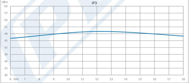
Click the following link (or enter part number in "SEARCH" on website) to obtain additional part information including price, inventory and certifications: 10 Watt P1dB, 6 GHz to 18 GHz, High Power Amplifier with Heatsink, SMA, 40 dB Gain, 46 dBm IP3 PE15A5050F
