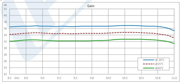
Click the following link (or enter part number in "SEARCH" on website) to obtain additional part information including price, inventory and certifications: 7 Watt P1dB, 8.5 GHz to 11 GHz, High Power Amplifier, SMA, 30 dB Gain, 46 dBm IP3, 5 dB NF PE15A5043
