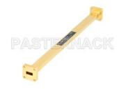
WR-42 Instrumentation Grade Straight Waveguide Section 9 Inch Length, UG-595/U Square Cover Flange from 18 GHz to 26.5 GHz
