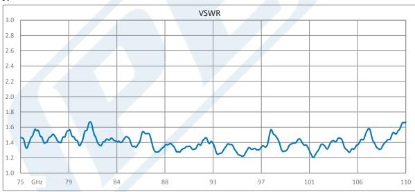
Click the following link (or enter part number in "SEARCH" on website) to obtain additional part information including price, inventory and certifications: WR-10 UG-387/U-Mod Round Cover Flange to 1.0mm Male Waveguide to Coax Adapter Operating from 75 GHz to 110 GHz PE-W10CA002
