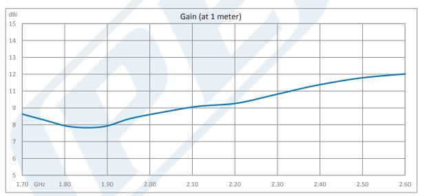
Click the following link (or enter part number in "SEARCH" on website) to obtain additional part information including price, inventory and certifications: WR-430 Waveguide Standard Gain Horn Antenna Operating From 1.7 GHz to 2.6 GHz With a Nominal 10 dBi Gain With CPR-430F Flange PE9864-10
